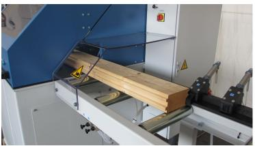
Outfeed table with pneum. stop faces for the workpiece positions, mounted on a ruler with metric scale (Option)
